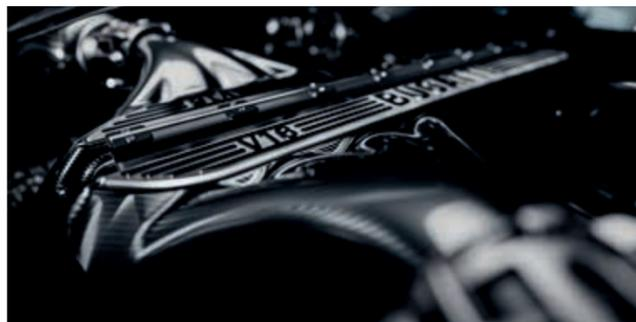
Bugatti Tourbillon : V16 Cosworth 8,3l - 1775bhp at 9000 rpm / 1775ch a 9000 tr/mn
